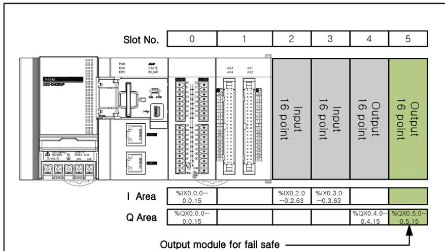
\* Equip output module for fail safe to last slot of system.
