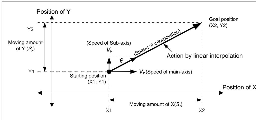
$$\text{Speed of sub}(V_y) = \text{Speed of main}(V_x) \times \frac{\text{Moving amount of Sub}(S_y)}{\text{Moving amount of Main}(S_x)}$$
