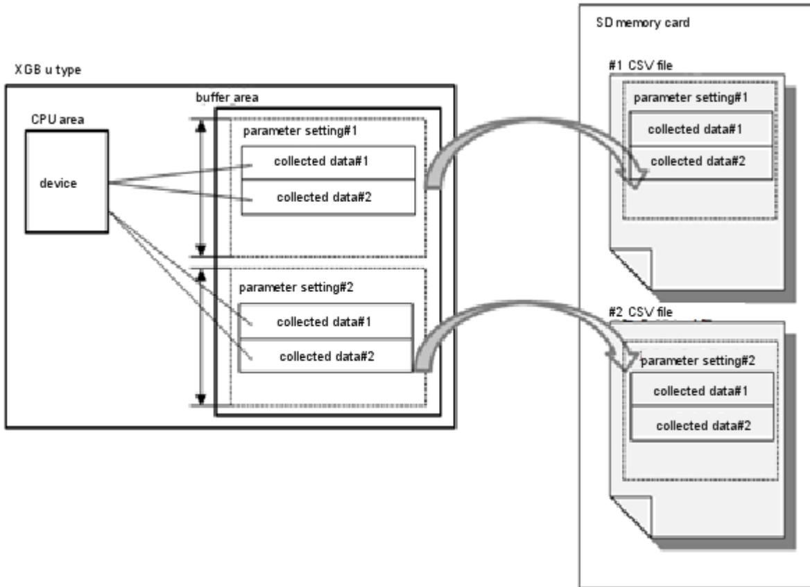
In accordance with the set sampling condition, the collected data are stored in the buffer memory first and then saved in to the temporary memory of the SD memory card when data log condition occurs. The size of buffer memory is fixed at up to 500KB per group. Therefore, setting too fast data sampling condition or sampling too much data, data loss can be caused by buffer memory excess. Data loss increases the DATA\_CLASH flag counter.
