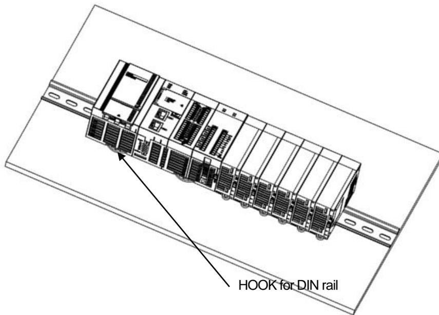
(b) In case of installing at panel
