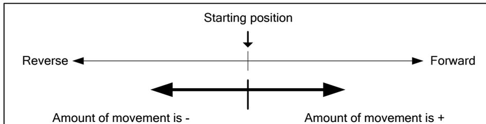
[Example] Set the Relative Coordinates as follow, Operate single-axis positioning control.
