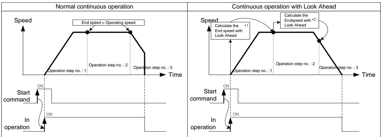
\*1 : moving amount of Step 2 and Step 3 is more than the deceleration stop distance from operation speed. So, endpoint speed = operation speed.
