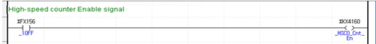
(d) To use additional functions of the high-speed counter, you need to turn on the flag allowing an operation command.
