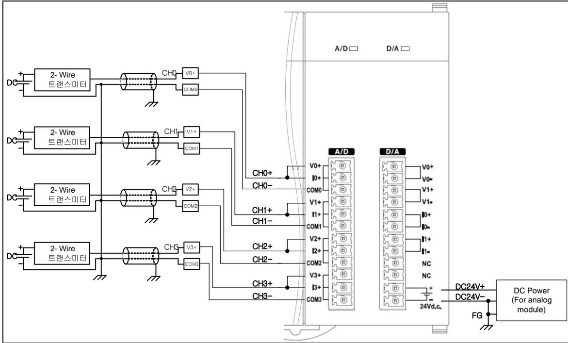
※ DC power for analog power supply have to connect DC24V- with FG.
