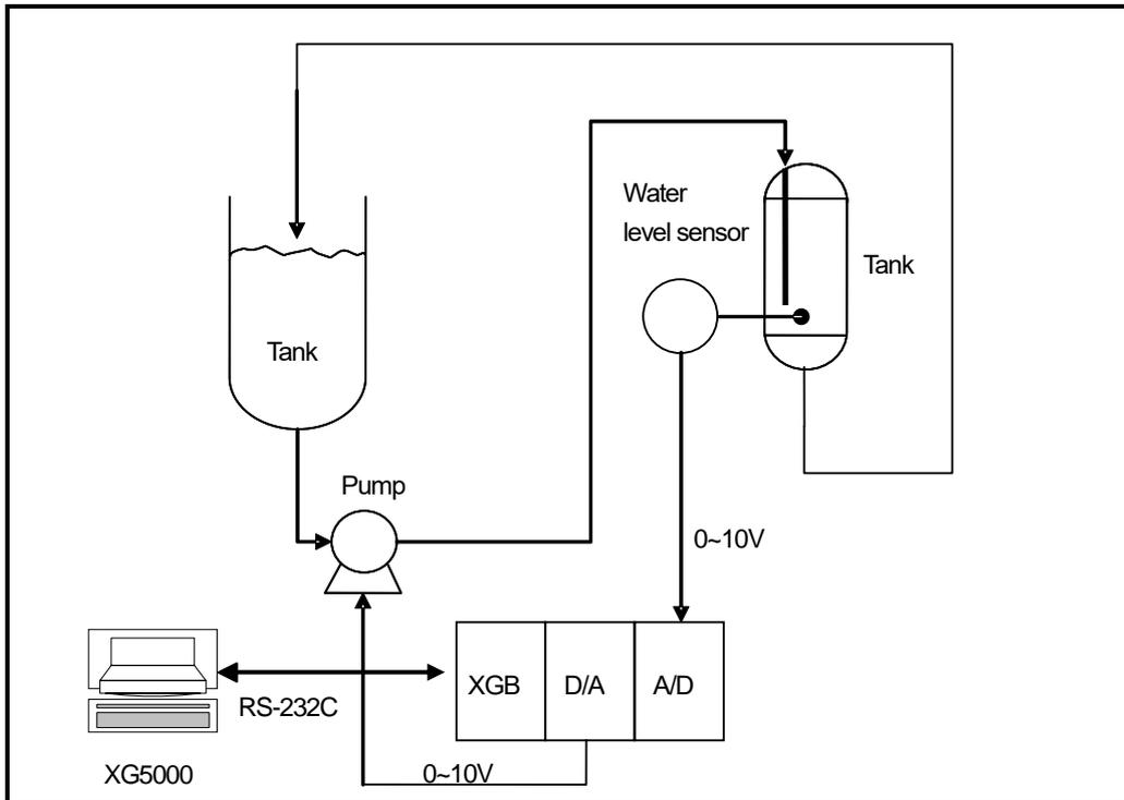
[ Figure 6.17 Example of water level control system ]
