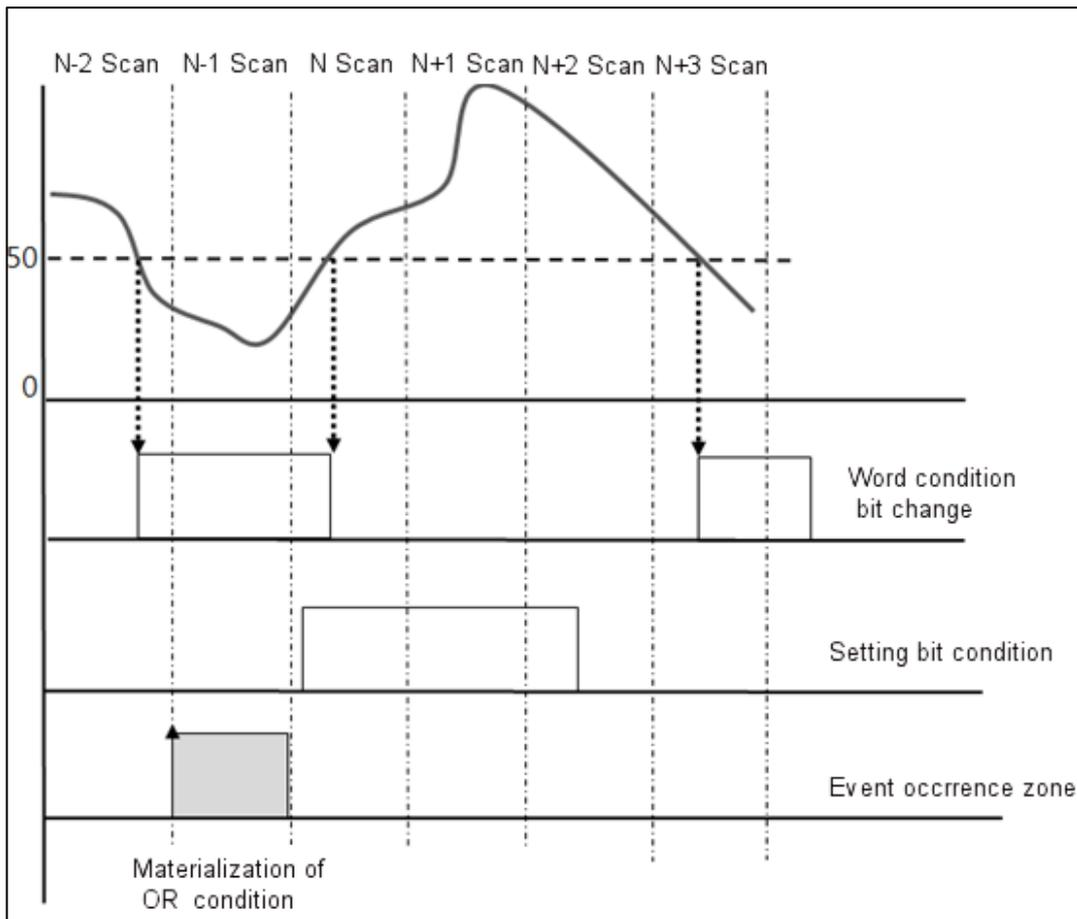
☞ When setting with combination of BIT and WORD conditions (release value set)
