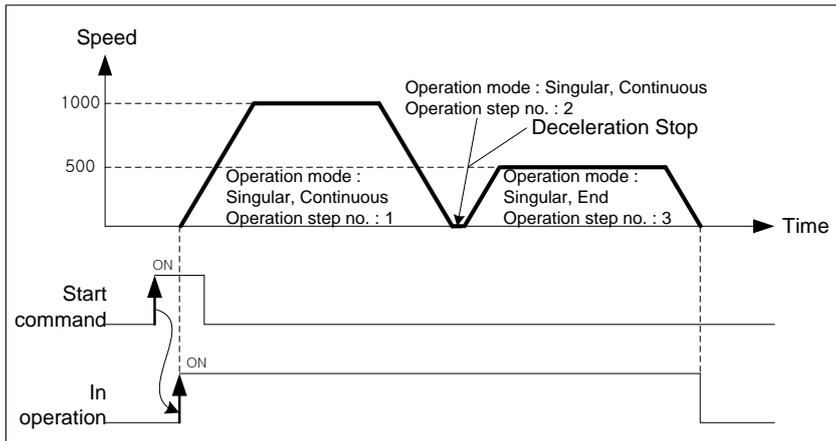
The Step1 will be operated by the start command. However, because the moving amount of next step is 0, it stops after deceleration, and then operates Step3 after 1 control period.
