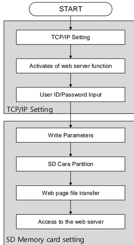
After setting the parameters of the embedded FEnet, you can access to the web server. In order to contact the web server, after connecting the PLC to Ethernet network, enter the IP set in XG5000 to the Internet Explore window.
