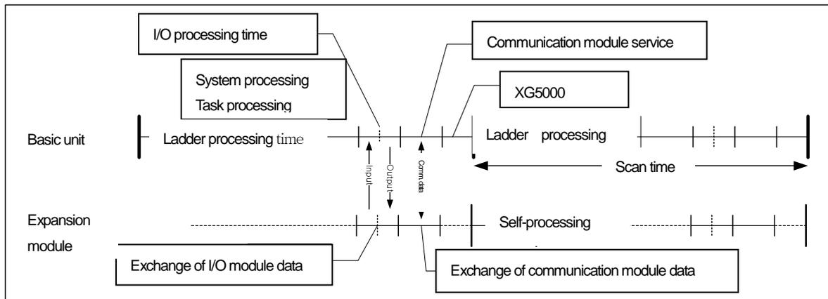
Scan time = Ladder running time + system processing time + digital module I/O processing time + analog I/O processing time + communication module processing time + XG5000 Service processing time
