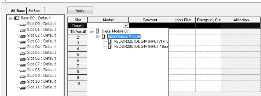
4) Double Click I/O Module. Select Pulse Catch output
