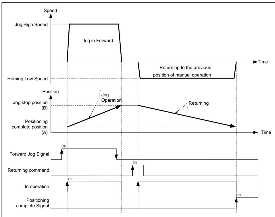
If value of the current position is "A" after positioning control operation and the positioning value changed by Jog operation is "B", execute positioning to "A" when executing the returning to the previous position of manual operation.
