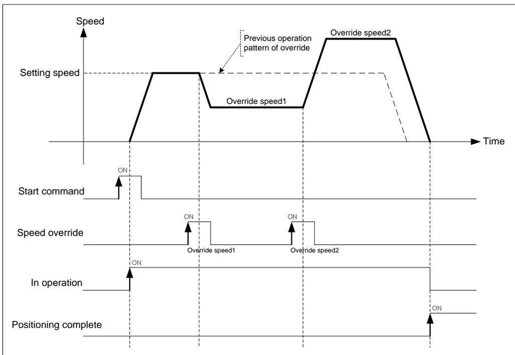
If you want to change the operation speed of positioning control in the current operation, you can change the operation speed by using the speed override command.
