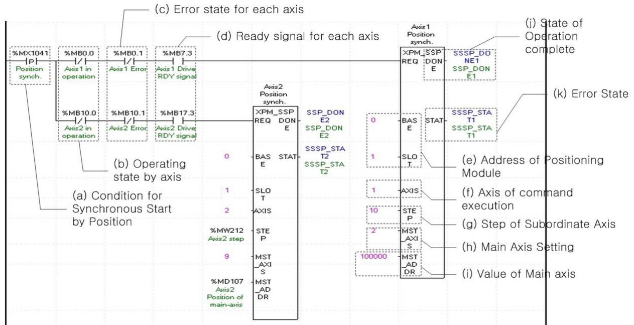
(a) This is the condition for Synchronous Start by Position
