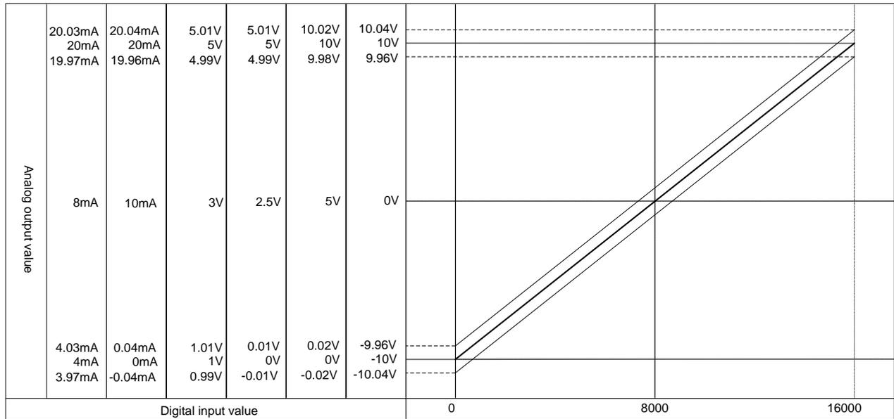
(1) Accuracy when using -10~10V output
