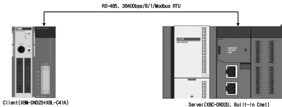
[Figure 2.11.2] XGT Modbus communication system configuration example
