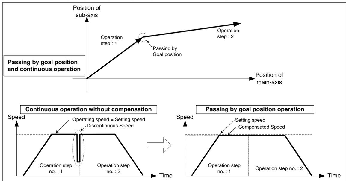
It decrease speed of acceleration, constant speed section as much as remaining amount of movement at the last section of current step to compensate position if operates as passing goal position operation.
