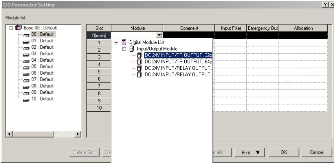
4) After setting I/O module, click Input Filter.
