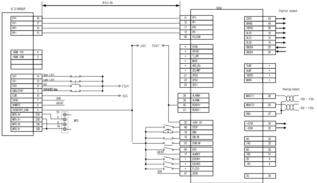
Note 1) Input signals DI1 to DIA and output signals DO1 to DO5 are default signals allocated by the factory.
