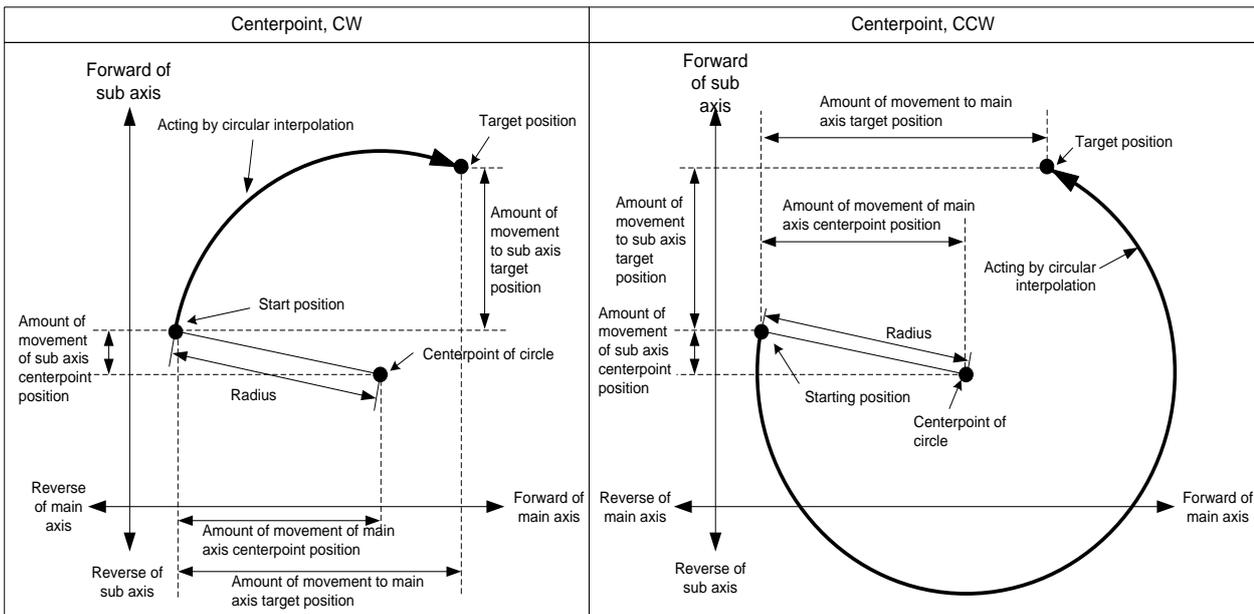
(c) If set target position of main axis and sub axis as “0”, than starting position will be same with target position and can progress circular interpolation that it is drawing circle. The radius of the circle is distance from starting position to center-point.
