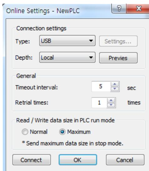
(c) After choosing the connection method with the PLC to be deleted, if you click 『Access』 or 『OK』 , all PLC programs, parameters, data, passwords will be deleted.
