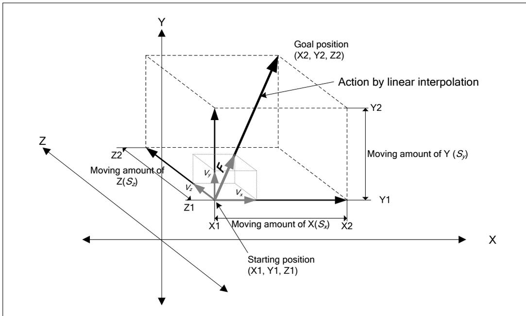
$$\text{Speed of sub}(V_y) = \text{Speed of main}(V_x) \times \frac{\text{Moving amount of Sub}(S_y)}{\text{Moving amount of Main}(S_x)}$$
