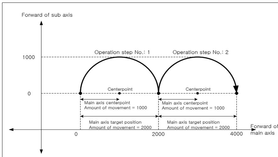
(3) Circular interpolation control which radius of starting point is different with radius of ending point.
