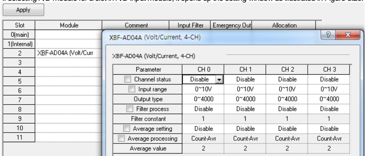
[ Figure 6.20 A/D input mode setting window ]
