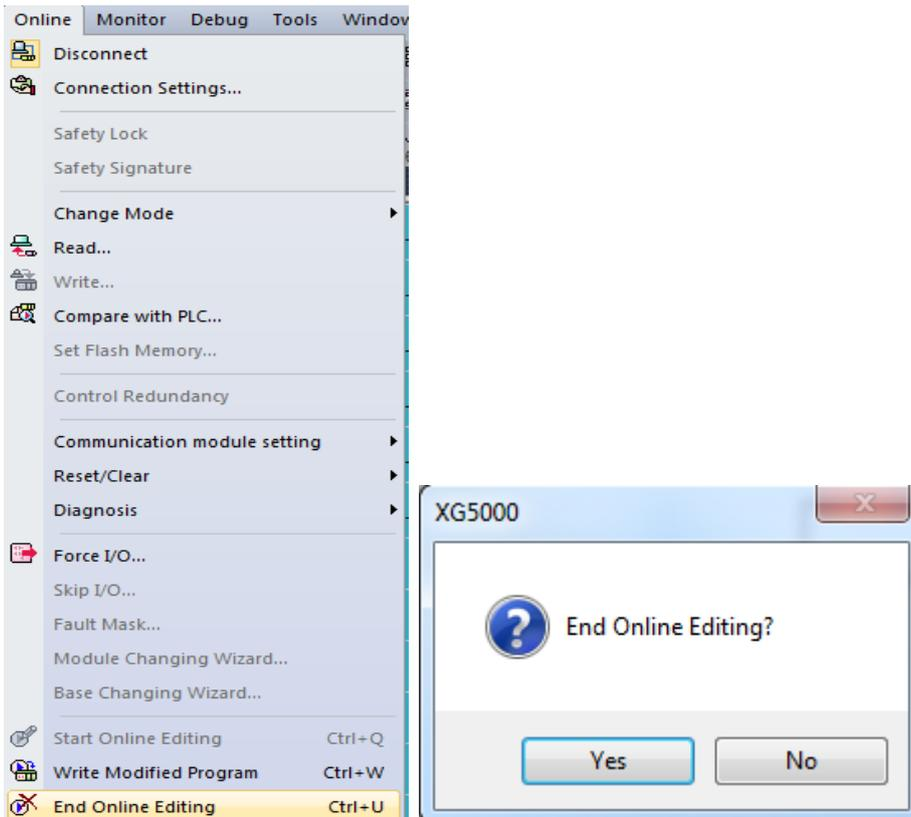
(7) The background color of the program window changes into the original one and modification during RUN is completed.
