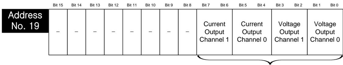
Interpolation time setting (2 bits per channel)
