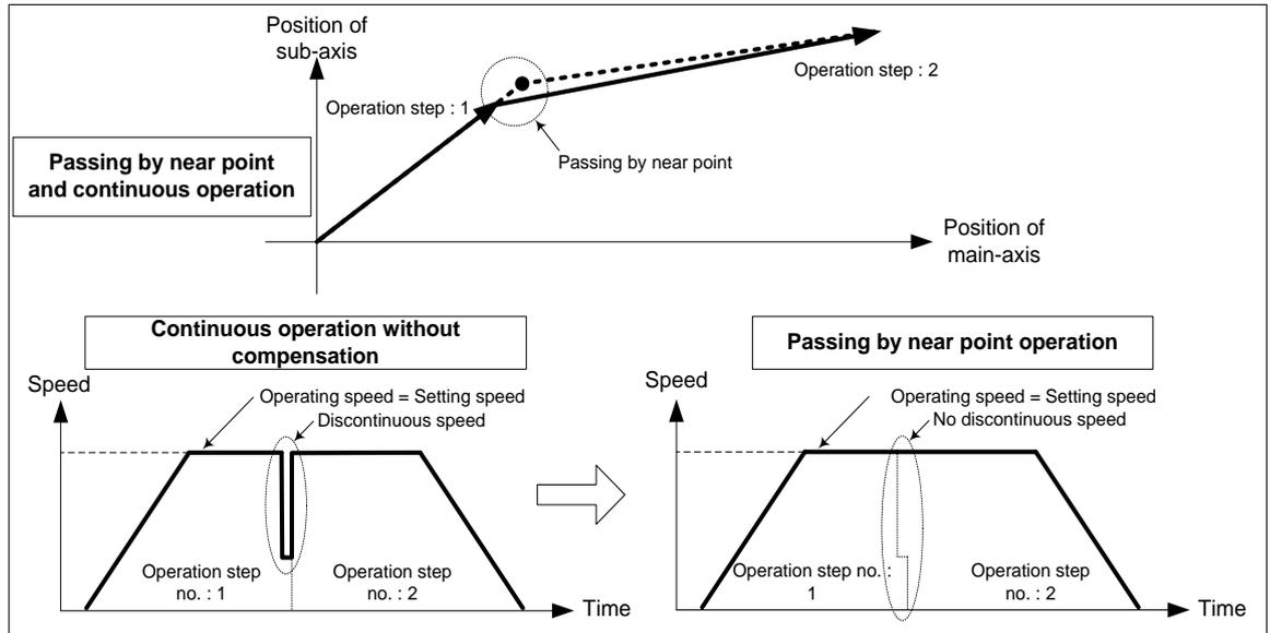
In the picture above, during general Continuous Operation, Occurring speed discontinuity because of remaining amount of movement at the last operation step NO.1. 「Near Passing」 Continuous Operation, you can move the remaining amount of movement to next step and execute Continuous Operation without speed discontinuity.
