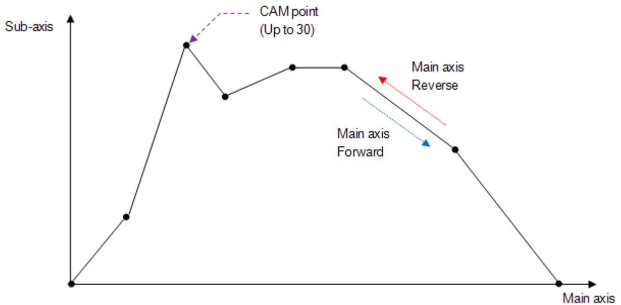
Like figure above, you can set up maximum 30 CAM data points, and it operates CAM curve between CAM points with straight line. CAM point data is set up at sub-axis and as type of (main-axis position, sub-axis position). CAM data point can be saved at the specified memory address of each axis by using "Write Variable Data" (XVWR, XPM\_VWR) command. For memory address to save CAM data point of each axis, refer to 3.10 User CAM data memory address.
