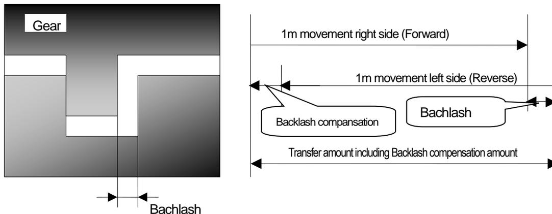
(e) It compensates by adding backlash compensation pulse to current output pulse within speed limit.
