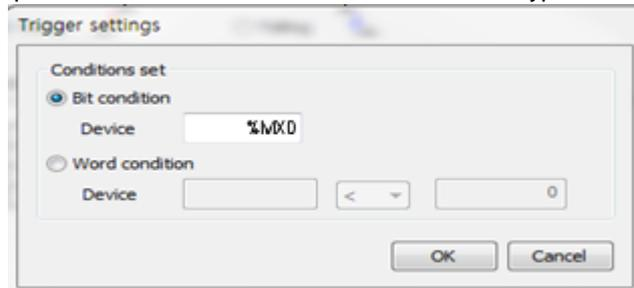
When setting is complete, the window closes and the conditions initially set at the Trigger Setting Condition menu are displayed as follows.
