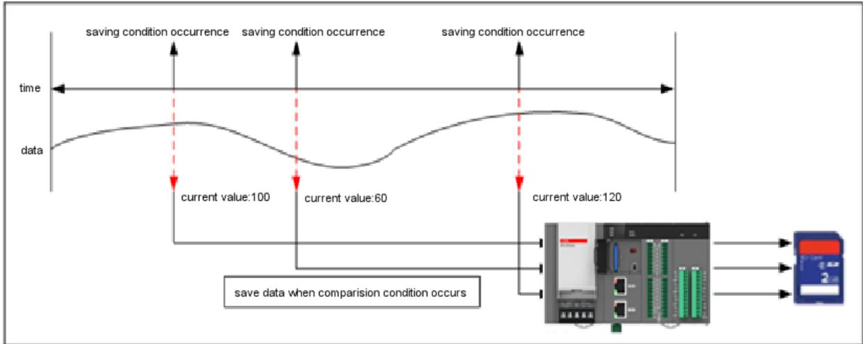
The collected data at each set cycle are scan END processed and saved into the SD memory as a CSV file.
