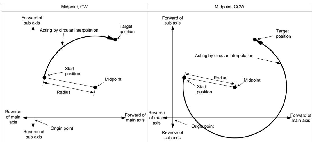
(c) If target position is same with start position, can progress circular interpolation. And the circle radius is distance from midpoint to starting position (=target position)
