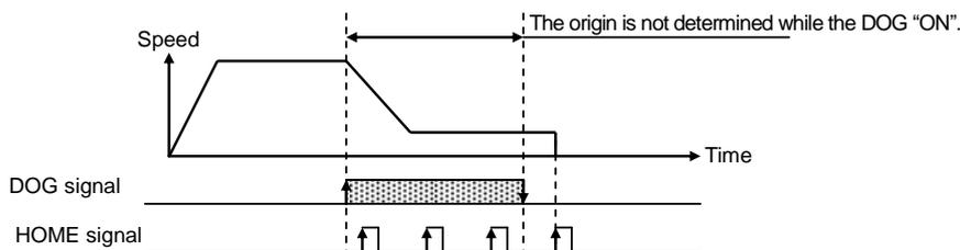
2. While the homing speed acts to the deceleration section by homing high speed after the DOG signal is changed from "Off" to "On", from "On" to "Off", the origin will not be determined even if encounters the HOME input.
