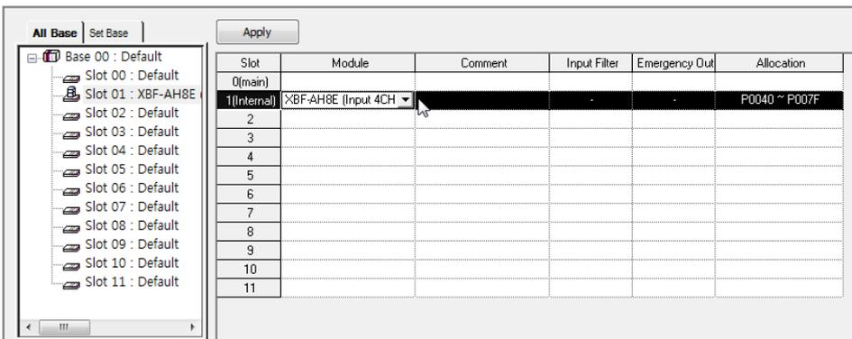
(6) A screen will be displayed for you to specify parameters for respective channels as below. Click a desired item to display parameters to set for respective items.
