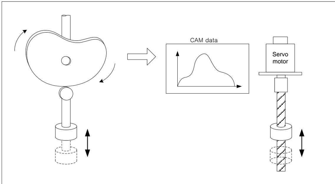
(b) You may write max. 9 CAM data blocks and apply it to each axis.
