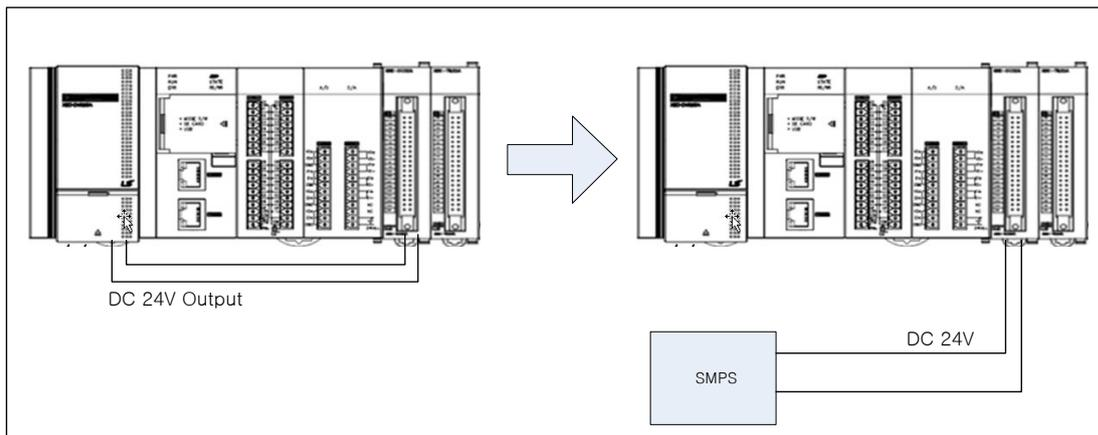
(5) AC110V/AC220V/DC24V cables should be compactly twisted and connected in the shortest distance.
