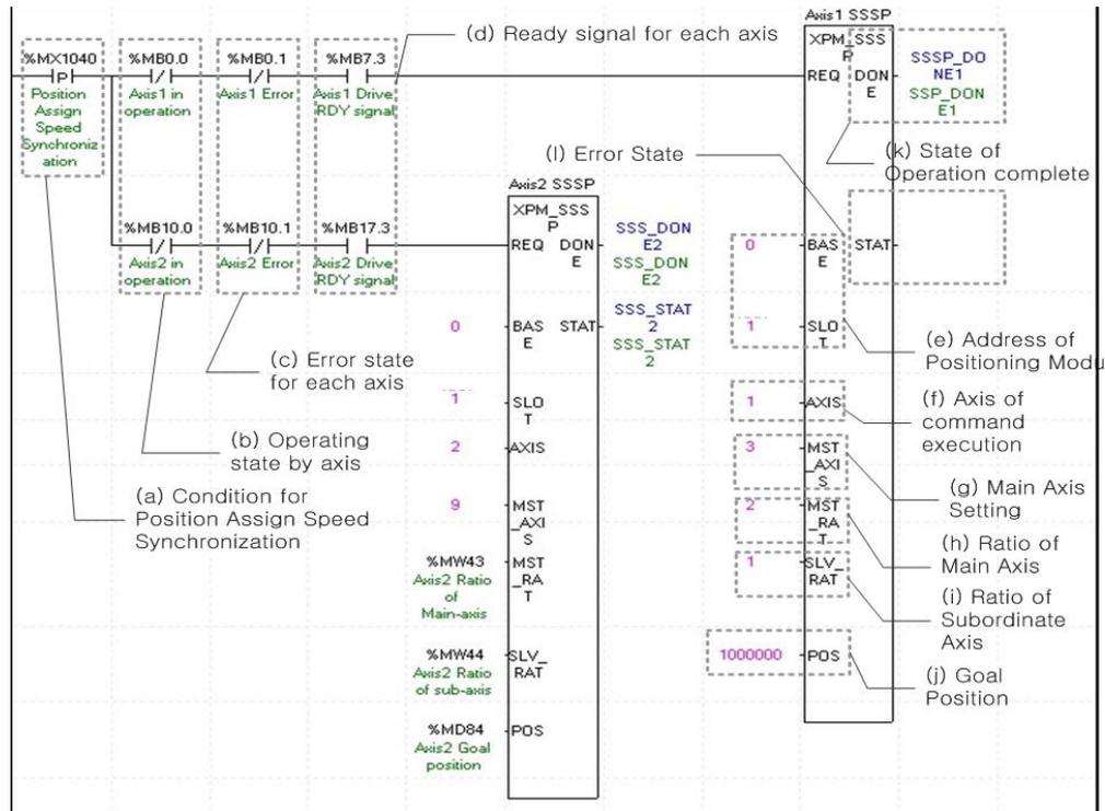
(a) This is the condition for Position Assign Speed Synchronization
