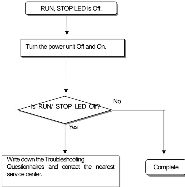
**6.2.4 Troubleshooting flowchart used when the I/O part doesn't operate normally.**
