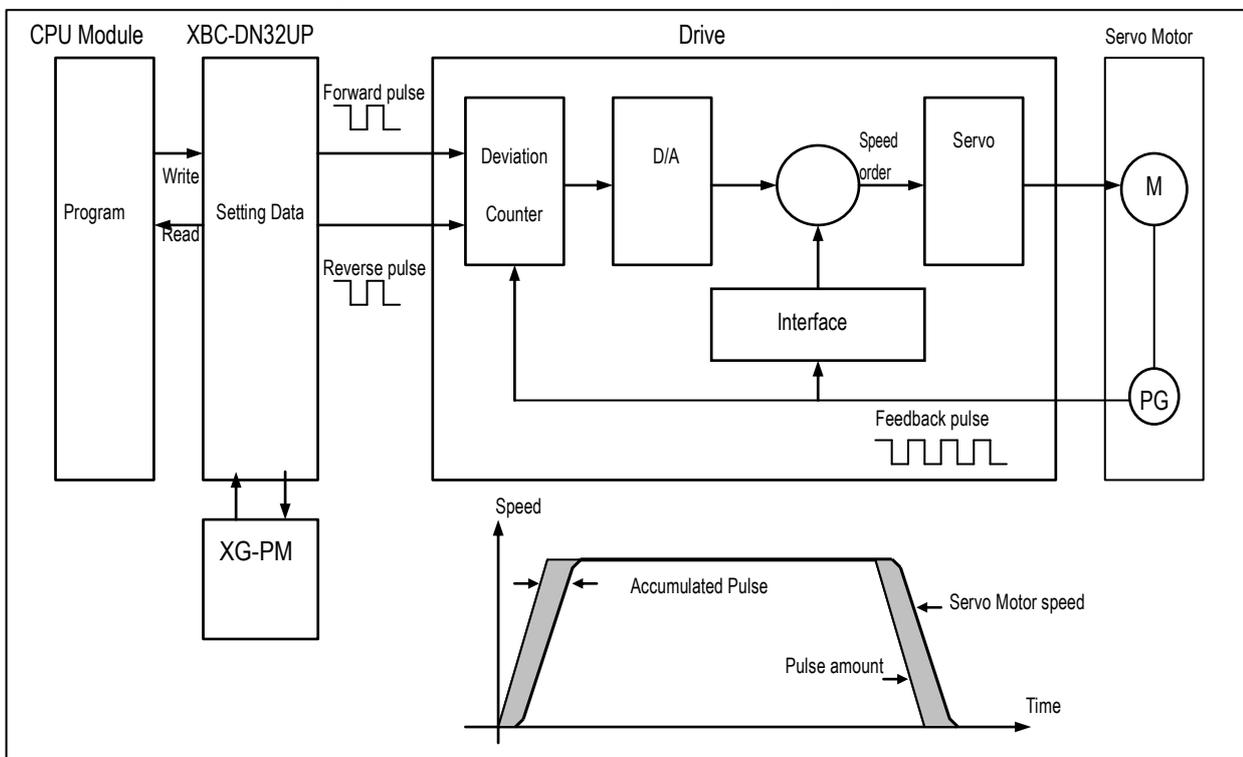
Fig. 1.2 Overview of Position Control for Servo Motor
