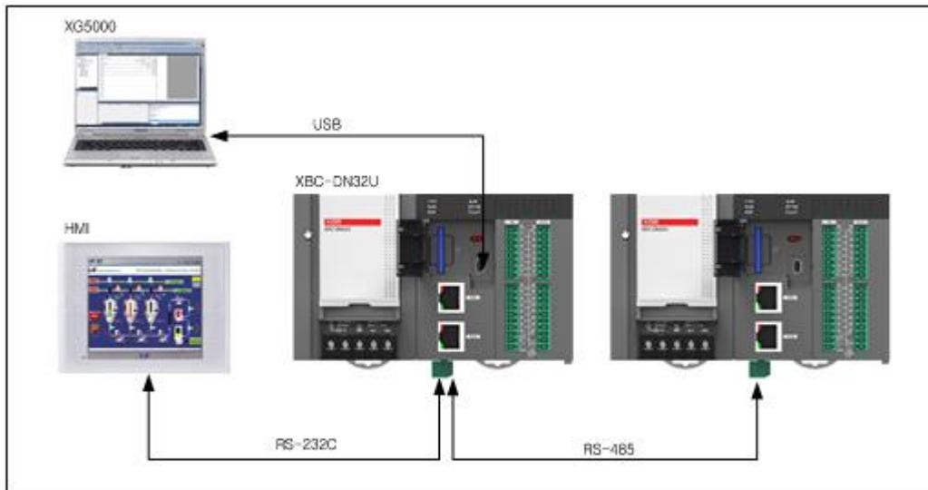
(3) Configuring 1:N communication system with the maximum 32 stations by using the basic unit's embedded RS-485 port
