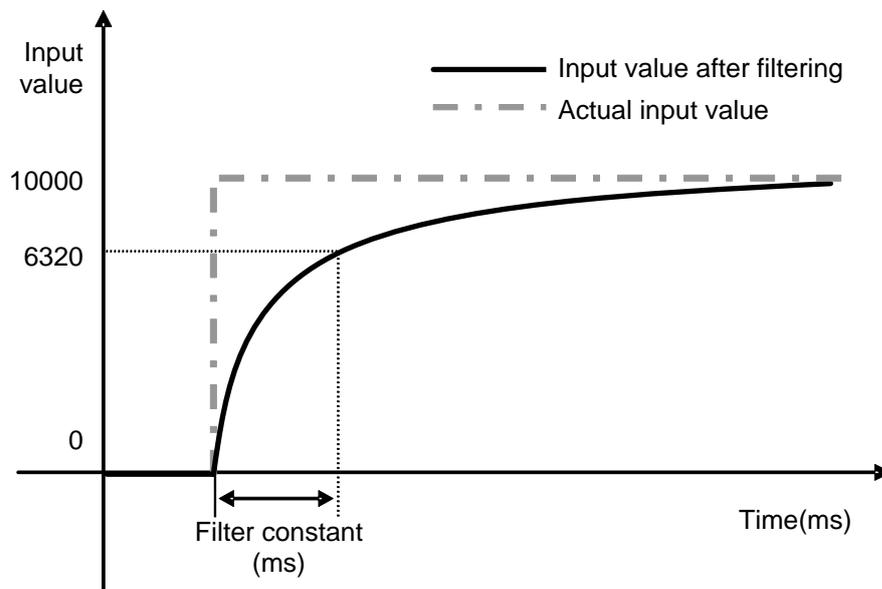
As the above graph, if the input value rapidly decreases from 0 to 10,000, the input value will be filtered. Specified time with filter constant is that the input value is the time to change by 63.2% of actual time constant.
