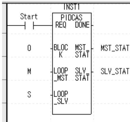
Cascade control is called a control method which is intended to increase control stability through quick removal of disturbance by connecting two PID control loops in series and is structured as follows.
