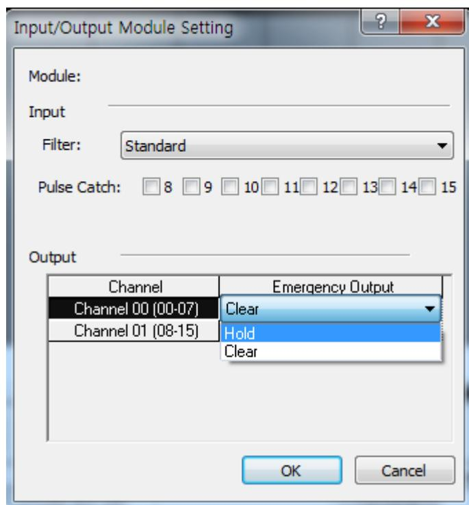
If setting Clear output will go off when error occurs, while If setting Hold output will go on.
