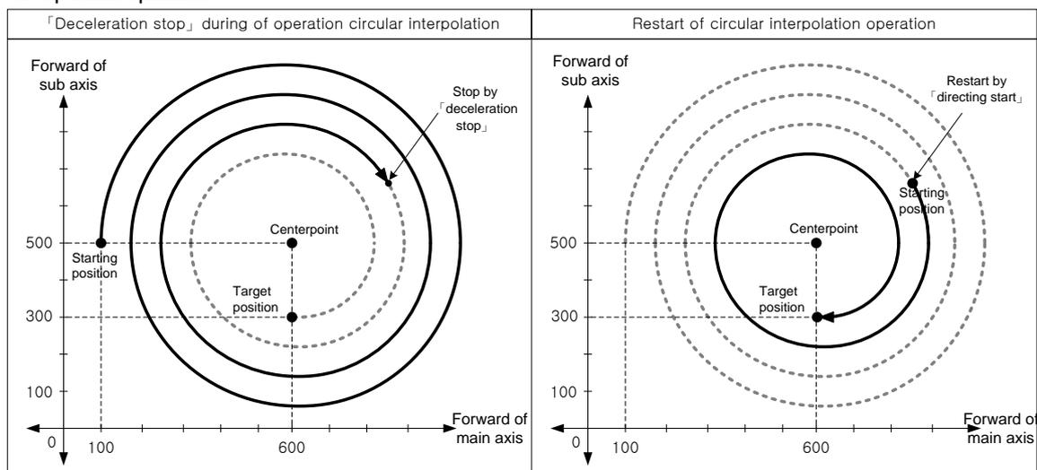
When decelerating in circular interpolation by dec. stop command and restart the same step no., not that executing circular interpolation after circular interpolation being executed 3 times, but that positioning at the goal position after going around 1 time, because 2 times of circular interpolation was executed in former operation.
