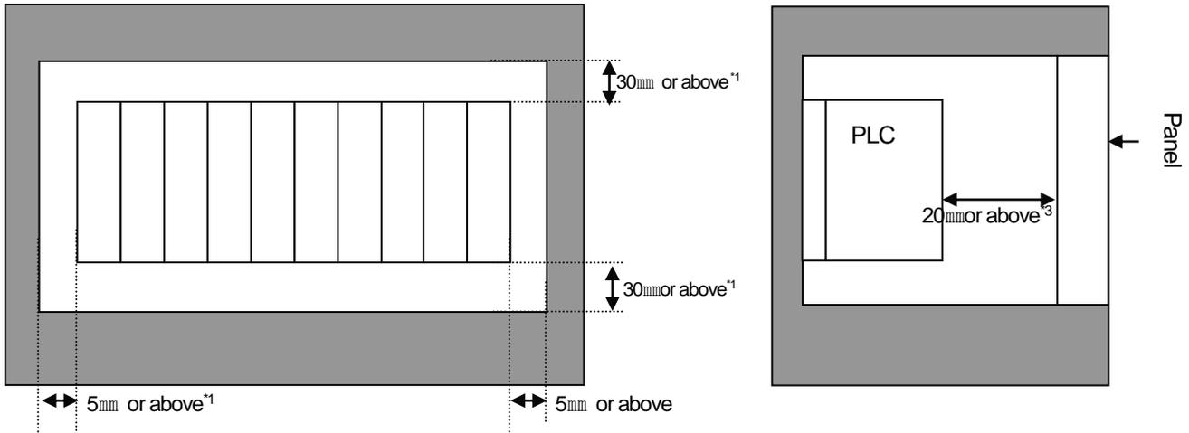
\*1 : In case height of wiring duct is less than 50 mm (except this 40mm or more)
