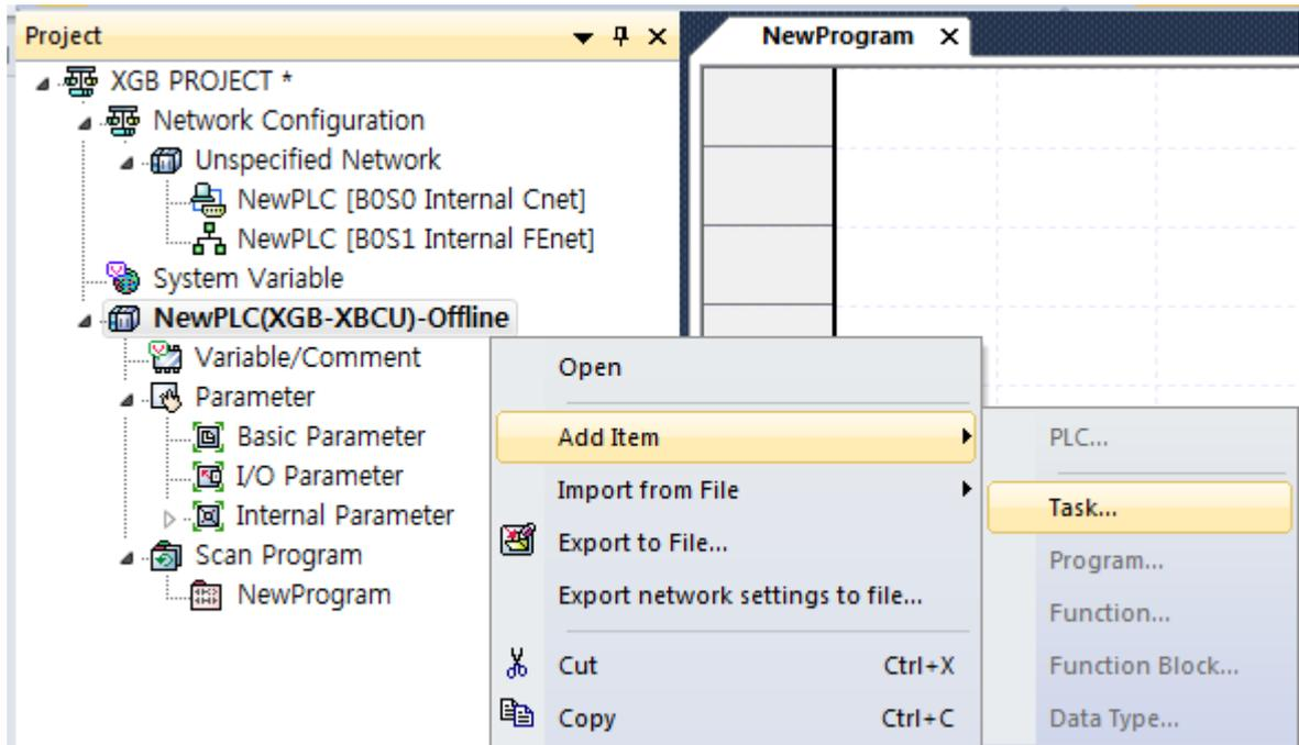
(b) The screen for registering the task will be displayed. Click 『External contact』 in the execution conditions and after entering the task name, input the items required for setting as below.
