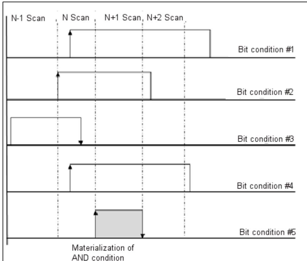
☞ When setting with combination of Bit and WORD conditions (no release value set)
