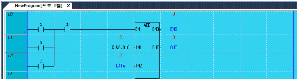
(5) When the modification of the program is completed, click 『Online』 - 『Write Modification During RUN』
