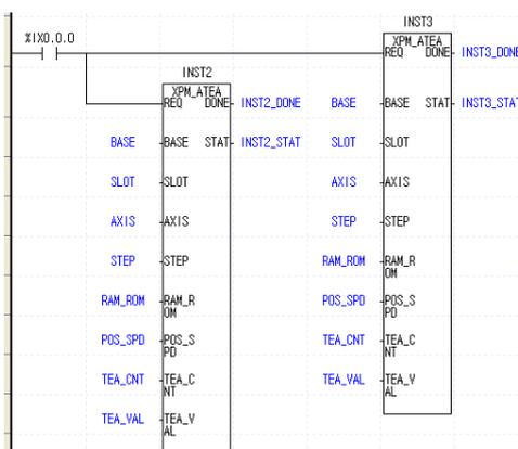
▷ For the different axes, you can simultaneously execute the same function blocks.
