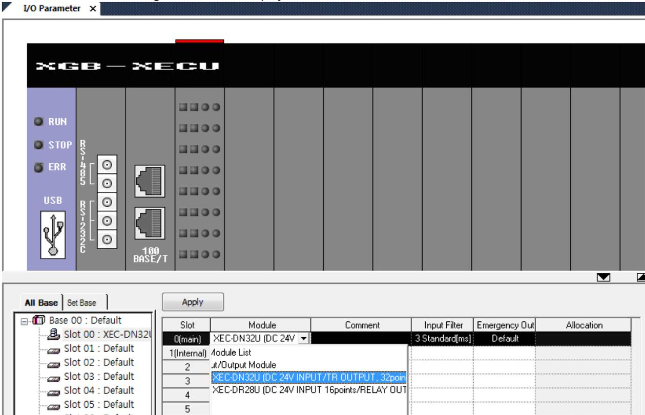
If you click the 『Module』 in the 『slot』 position, the list of each module will be displayed. Then, choose the module that is matched with the actual system to be configured. The selected slot will be displayed as below.
