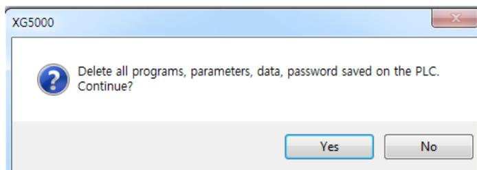
(b) If you choose 『Yes』 in the dialog box, the window for selecting the connection method with the PLC to be deleted is created.
