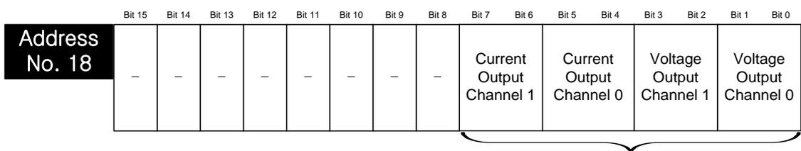
Interpolation method setting (2 bits per channel)
