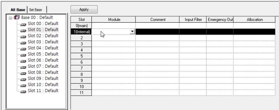
(4) Click the arrow button on the screen above to display the screen where an applicable module can be selected. Search and select the embedded analog input/output module to select.
