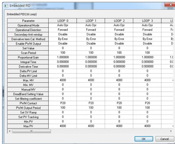
[ Figure 6.8 Built-in PID function parameters setting window ]
