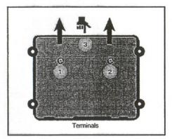
Remove the two screws 1 & 2 (shown in the diagram above) from the base of the VCD Drive. Lift the printed circuit board assembly at point 3 and slide it in the direction of the arrows.
