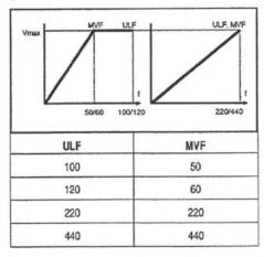
Factory setting: ULF = 100Hz, MVF = 50Hz
