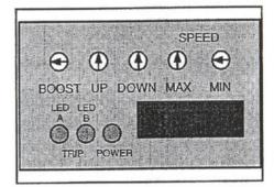
Ensure that **BOOST** and **MIN** are set fully anti-clockwise as shown above. Ensure that **UP**, **DOWN** and **MAX** are at mid-point as shown above.
