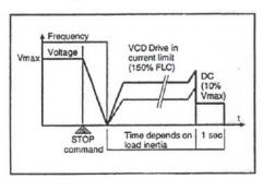
DC-Braking follows a pre-defined sequence as shown above. When a **STOP** command is received, the
