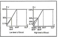
If the VCD Drive is configured for Fixed Boost and the motor fails to start, turn the **BOOST** preset clockwise to increase the starting torque. Boost should be set at the minimum required to start the motor under load. If the setting is too high, the motor may become over-heated.
