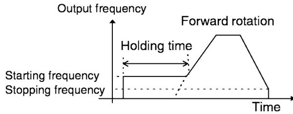
The operation does not start when the setting frequency is less than the stopping frequency.
