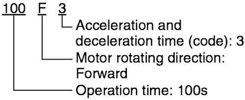
Set the operation time to 0.00 for stages not used, which are skipped in operation.
