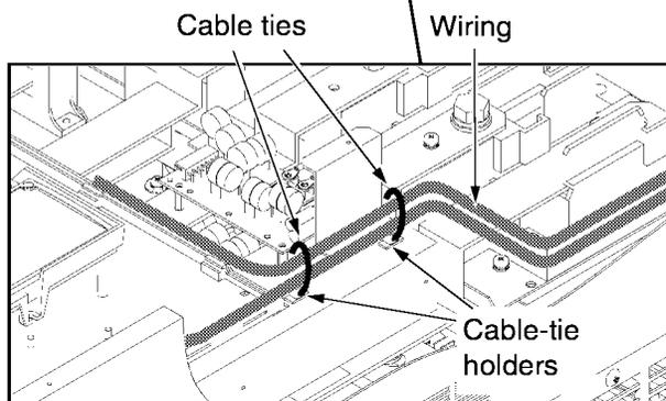
Figure 2-3-15 The securing points of the cables
