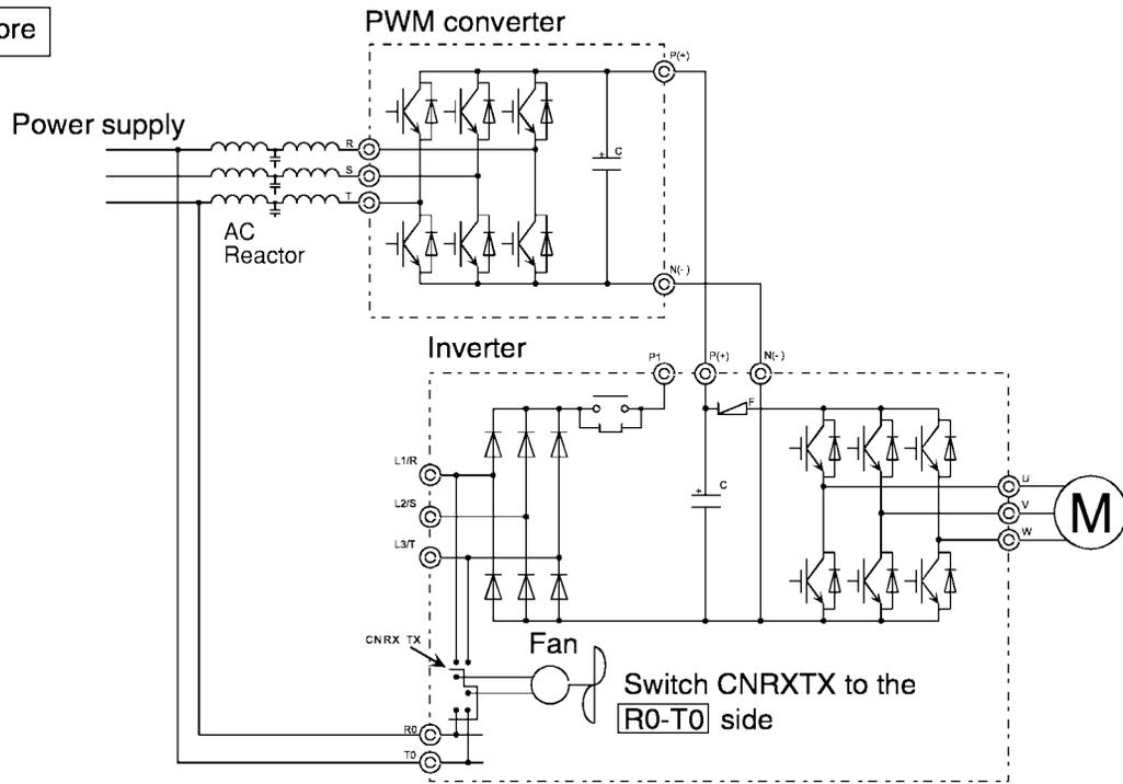
Figure 2-3-7 Example of connection by combination with power regeneration converter
