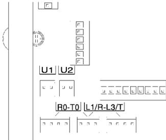
When shipped from the factory, CN UX is connected to the **U1** side and CN RXTX is connected to the **L1/R-L3/T** side.
