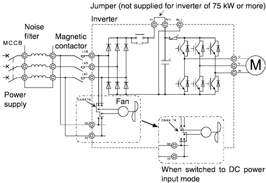
Figure 2-3-6 Fan power switching
