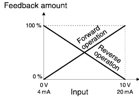
Only positive values can be input for this feedback amount of PID control. Negative values (e.g., 0 to -10 V, -10 to 0 V) cannot be input, thereby the function cannot be used for a reverse operation by an analog signal.
