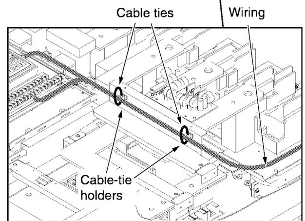
Figure 2-3-17 The securing points of the cables
