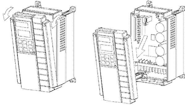
Figure 1-3-1 Removing the surface cover (for inverter of 22 kW or less)
