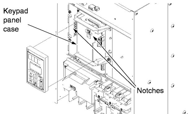
Figure1-3-4 Removing the keypad panel (for inverter of 30 kW or more)
