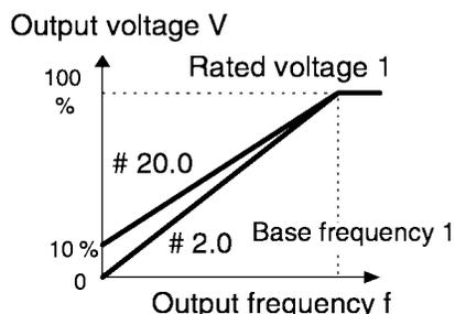
**Note:** As a large torque boost value creates overexcitation in the low-speed range, continued operation may cause the motor to overheat. Check the characteristics of the driven motor.
