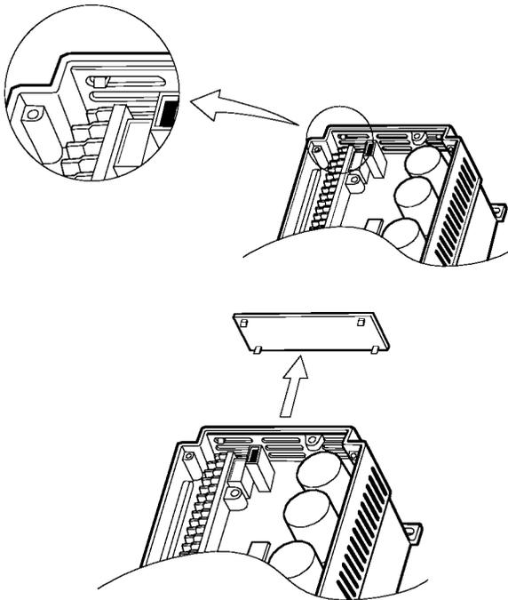
Figure 2-2-4 Removing the ventilating cover
