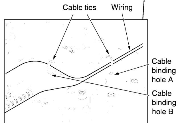
Figure 2-3-13 The securing positions of the control-circuit line of inverter
