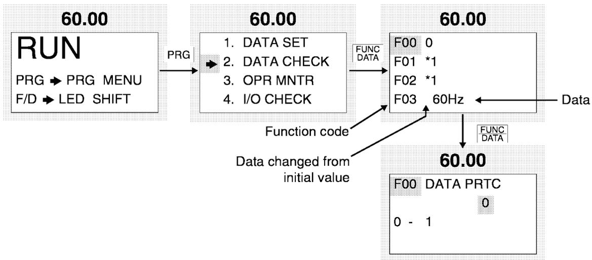
Select the desired function and press  $\boxed{\text{FUNC DATA}}$  to check the function data. By pressing  $\boxed{\text{FUNC DATA}}$ , the screen switches to the "DATA SET" screen, to modify data.
