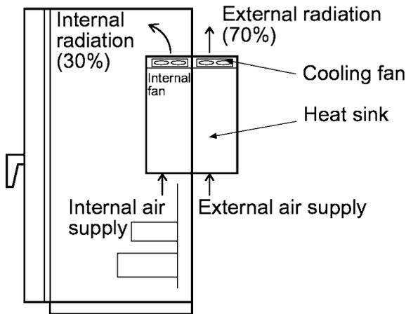
Figure 2-2-2 External cooling system
