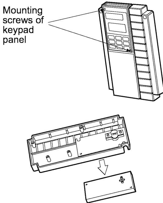
Figure 1-3-3 Removing the keypad panel
