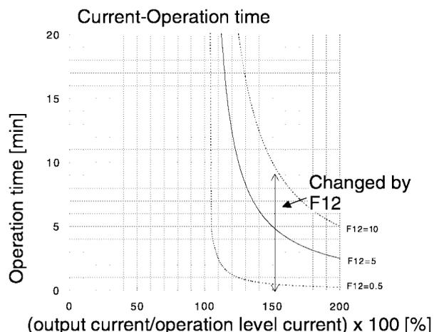
**F13 Electronic thermal O/L relay (for braking resistor)**
