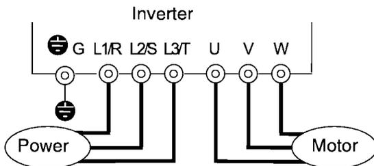
Figure 3-1-1 Inverter connection
