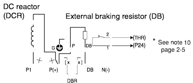
Figure 2-3-4 Connection (7.5 kW or less)
