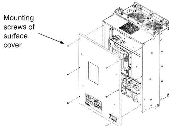
Figure 1-3-2 Removing the surface cover (for inverter of 30 kW or more)
