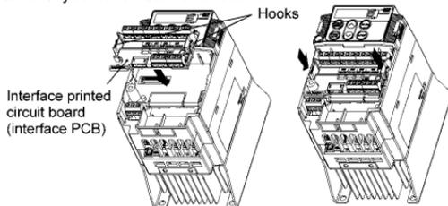
Figure 2.21 Mounting the Interface Printed Circuit Board (Interface PCB)
