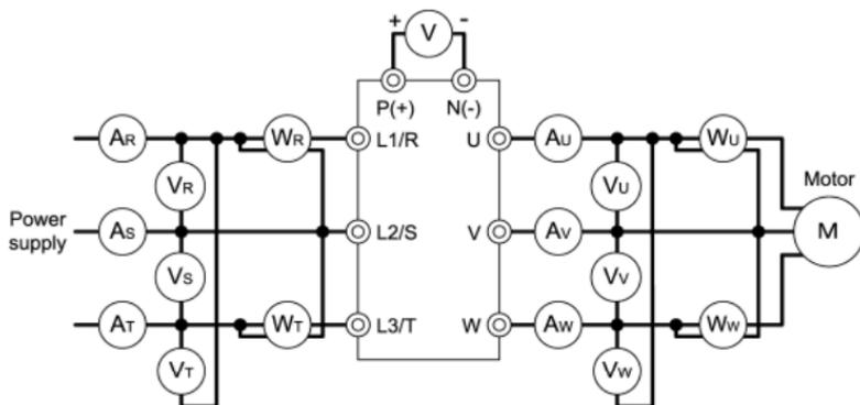
Figure 7.1 Connection of Meters
