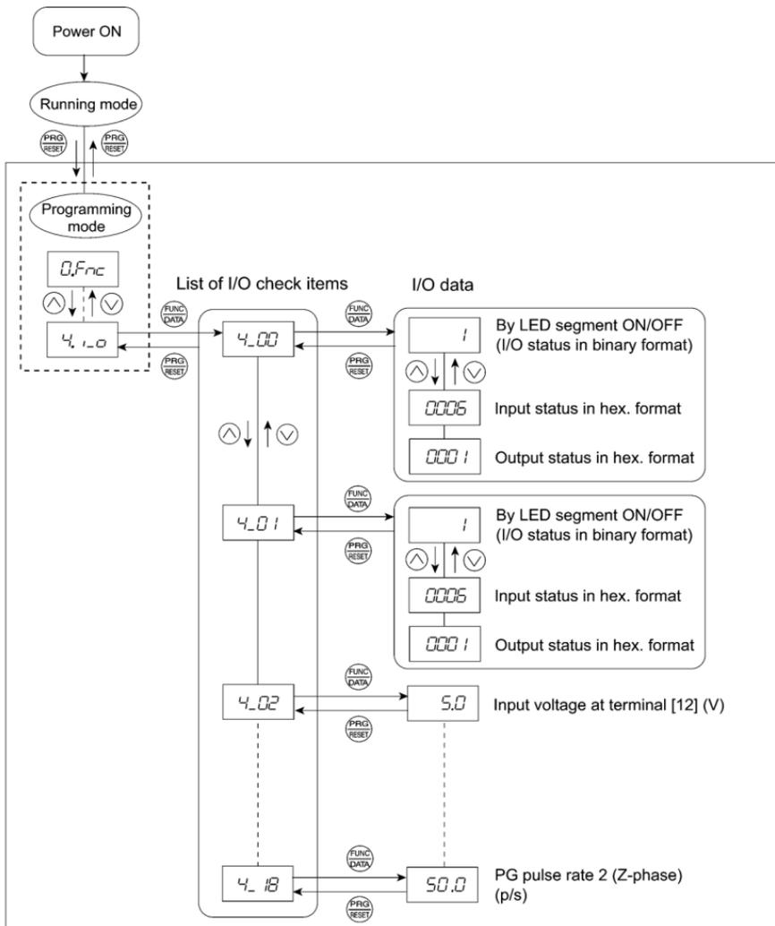
Figure 3.5 Menu Transition in Menu #4 "I/O Checking"
