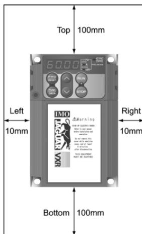
Figure 2.1 Mounting Direction and Required Clearances
