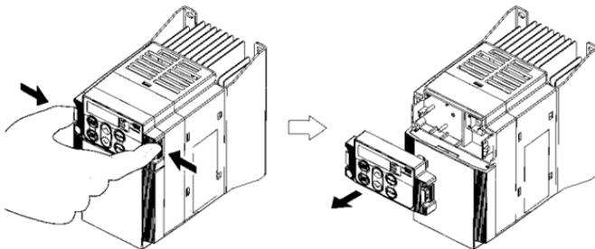
Figure 2.25 Removing a Keypad
