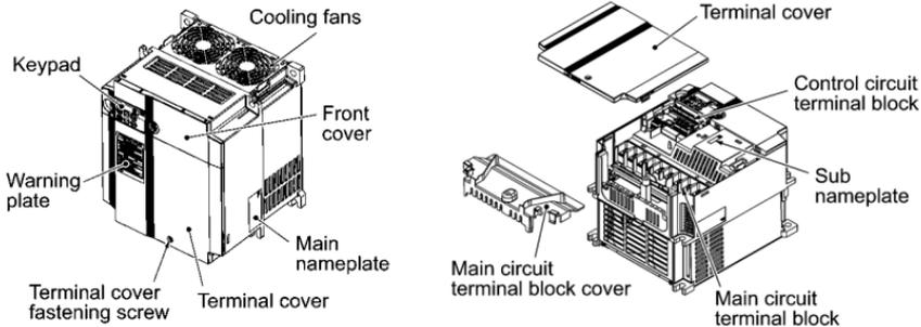
Figure 1.2 Outside and Inside Views of Inverters (VXR60A-2)
