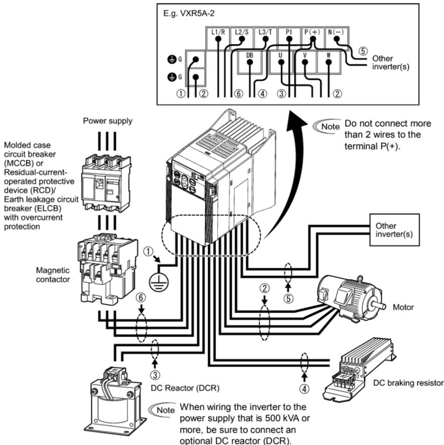
Figure 2.9 Wiring Procedure for Peripheral Equipment
