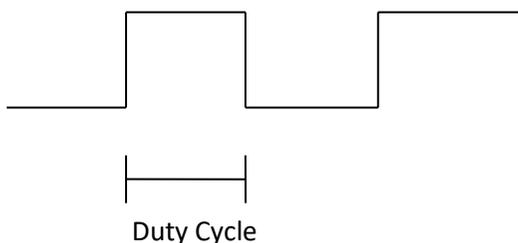
At controller power-up or during a download, the PWM output is maintained at zero until both the Period (count) and the Duty cycle (count) are loaded with non-zero values. When the controller is placed in stop mode, the state of the PWM outputs is dependent on the *PWM State on Controller Stop* configuration.
