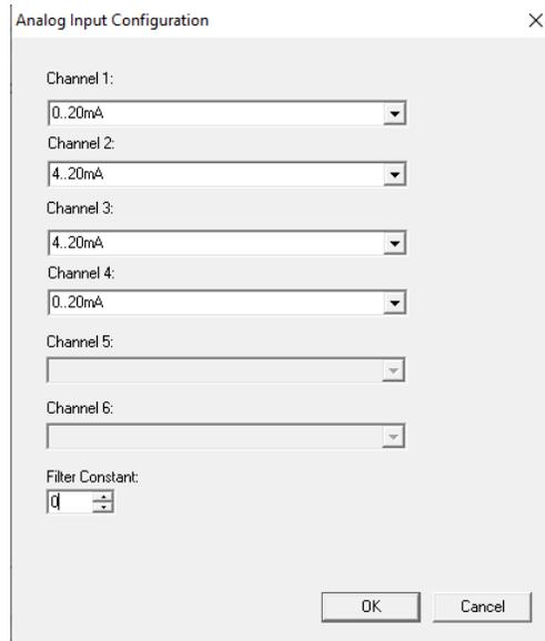
Figure 14.10– Analogue Input Configuration Dialog
