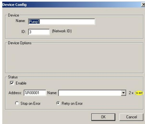
This configuration is reached from the Device List when adding or modifying an existing device.
