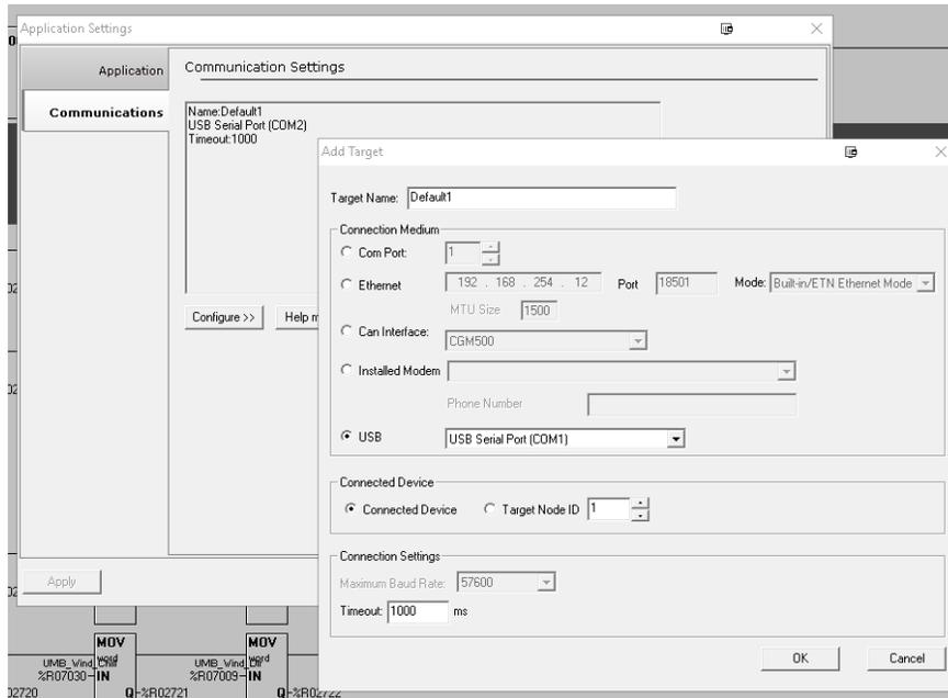
Figure 14.6 – Add Target Screenshot in *i3 Configurator*
