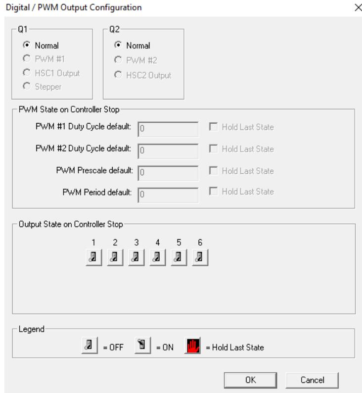
Figure 14.9 – Digital / PWM Output Configuration Dialog
