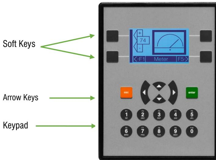
Figure 12.1 – Types of Keys and Buttons
