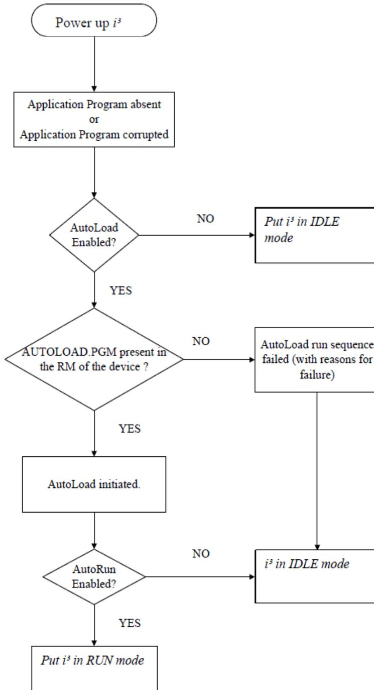
Figure 15.7 – Flow Chart for AutoLoad
