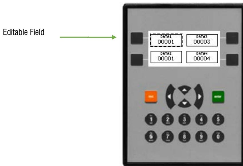
Figure 12.2—i<sup>3</sup>A Lite and Editable Field
