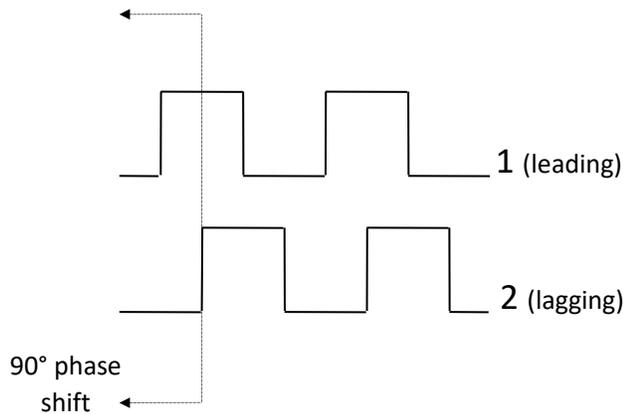
Using the above waveforms and a HSC input configuration of “Quadrature” - “1 leads 2, count up,” the accumulator will count up when 1 is rising and 2 is low, 1 is high and 2 is rising, 1 is falling and 2 is high, and when 1 is low and 2 is falling. This results in 4 counts per revolution. So, in order to determine the number of cycles, the accumulator would have to be divided by 4.
