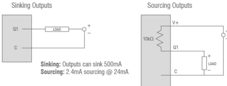
Figure 10.4 – Model -10D14: Sinking and Sourcing Outputs
