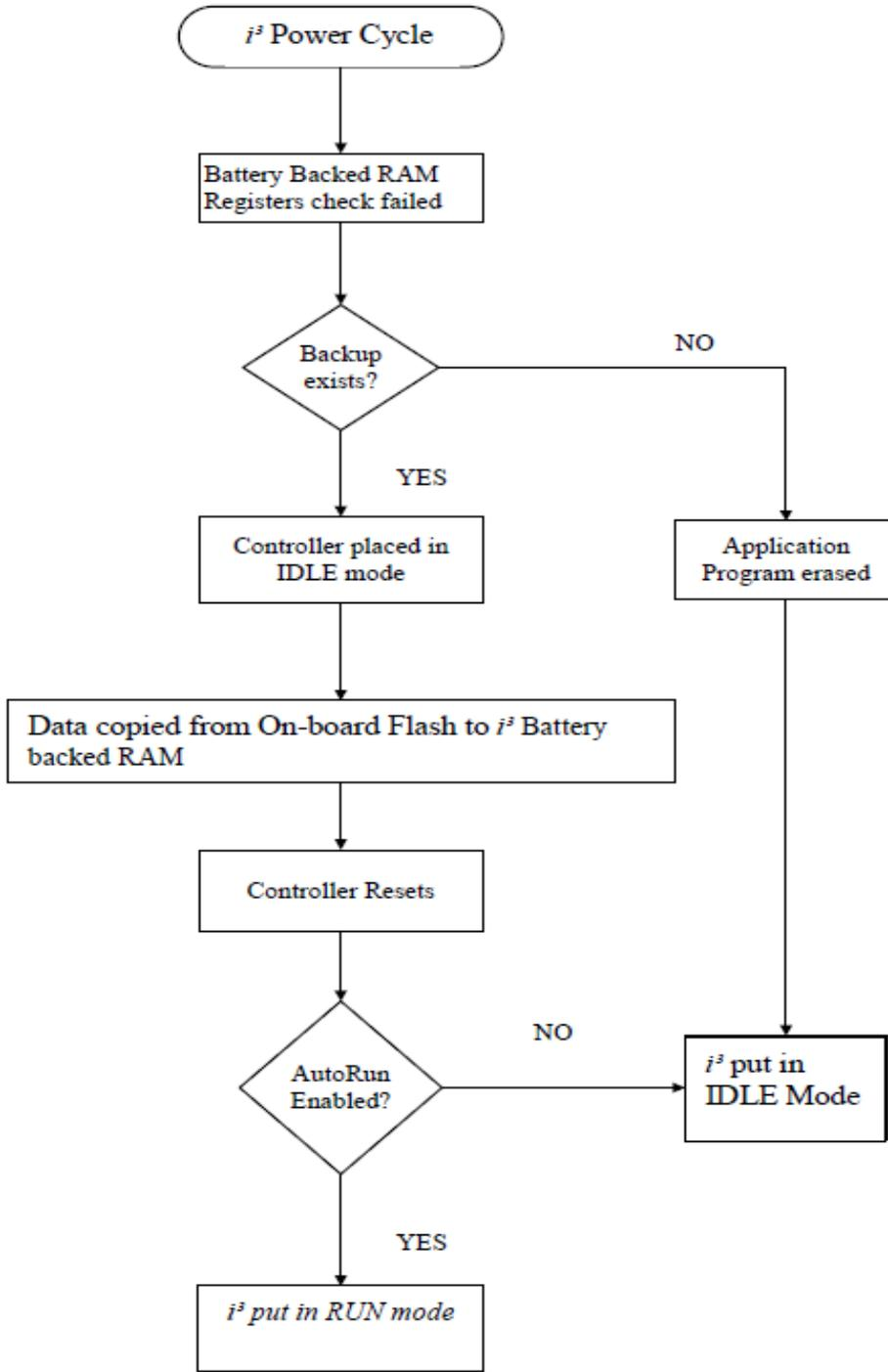
Figure 15.5 – Flow Chart for Automatic Restore
