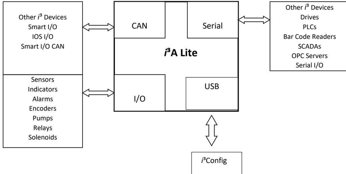
Figure 2.2 – Visual Overview of i<sup>3</sup>A Lite Connectivity
