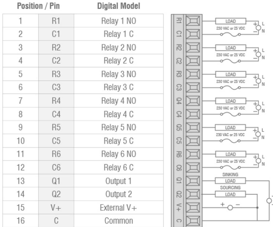
**NOTE:** Internal 10kΩ resistors between: V+ and Q1; V+ and Q2
