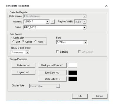
Select %SR047, RTC\_Date as the starting register to display the date.
