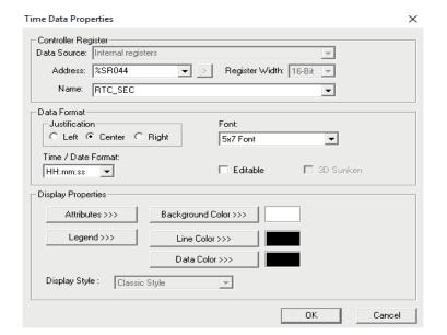
Enter the starting register as %SR044 and the next 2 registers will also be used. This will provide the hours, minutes and seconds for display.
